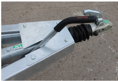
Couplings are AL-KO and KNOTT brand and they have brakes
